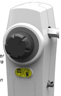
The High Flow system has a automatic push feature to continually dispense diluted chemical. There is a small plug with a lock symbol, when removed it allows the feature to operate. Push and twist the grey operating button clockwise to activate the feature. When the container is full push the operating button again to deactivate.
